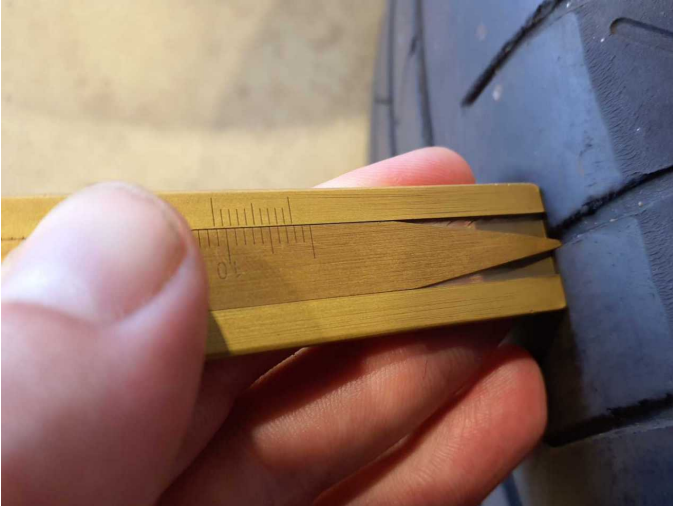
Damage 6: 2nd wheel set: 2 tyres - Worn - Replace
