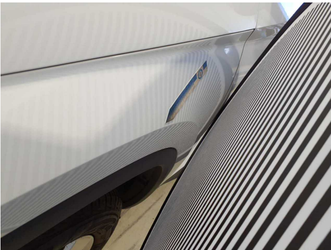
Damage 7: Mudguard - left side: Mudguard - left side - Dent / paintcoat damage - Repair and paint
