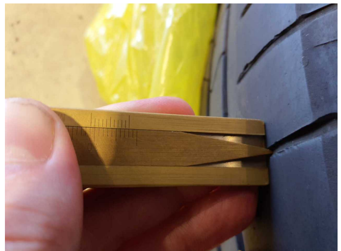
Damage 6: 2nd wheel set: 2 tyres - Worn - Replace
