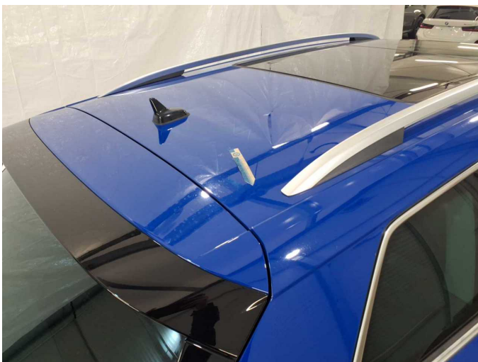
Damage 1: Roof: Roof - dent(s) - Smooth repair work
