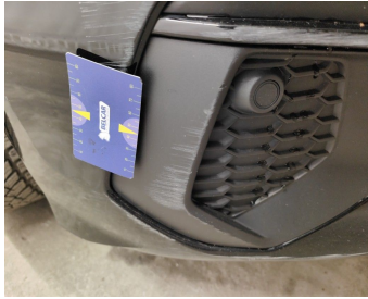
Bumper Front / Trim Right / Replace-scratch
