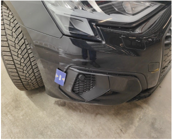
Bumper Front / Trim Right / Replace-scratch
