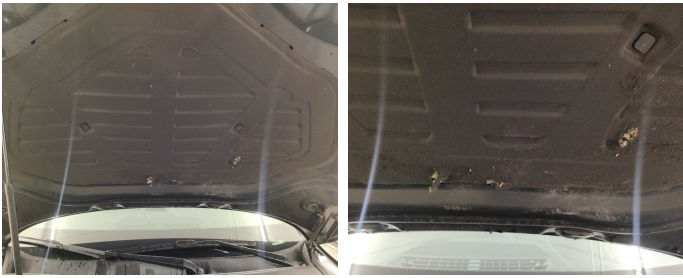
Front Bonnet / Insulation / Replace-cracked
