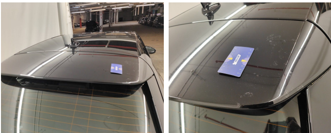
Rear Bonnet // Smart Repair Medium-Chemical reaction
