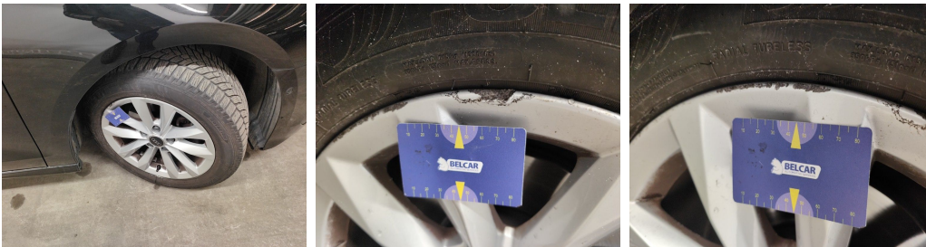
Wheel Alloy Front Right // Repair-scratch
