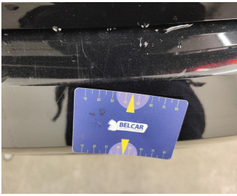
Bumper Rear // Painting-scratch
