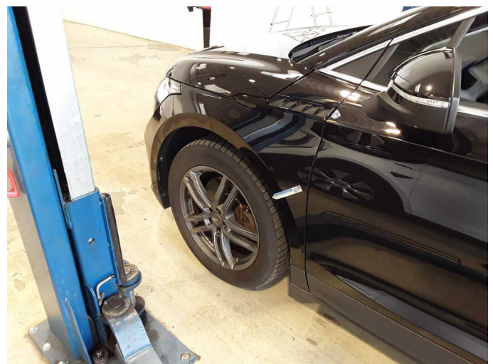
Damage 5: Mudguard - left side: Mudguard - left side - Dent / paintcoat damage - Repair and paint
