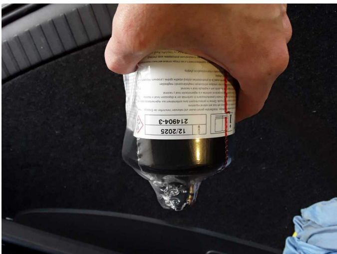
Damage 1: Equipment: Tirefit filler - Expired - Replace
