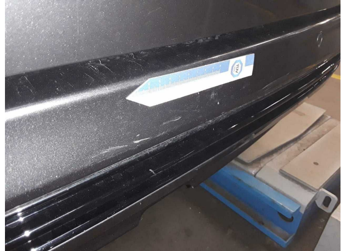
Damage 6: Rear bumper: Rear bumper - Dent / paintcoat damage - Paint
