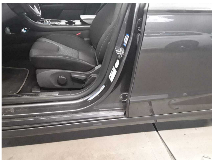
Damage 5: Body: B-pillar - left side - Dent / paintcoat damage - Repair and paint
