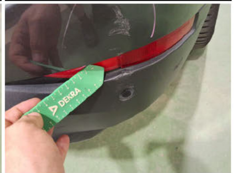
Reflector / Back Right / Broken
