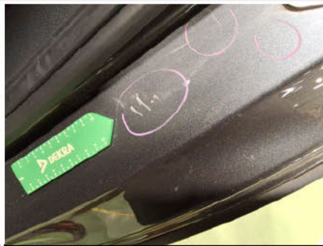
Door sill / Interior Back Left / Scratched
