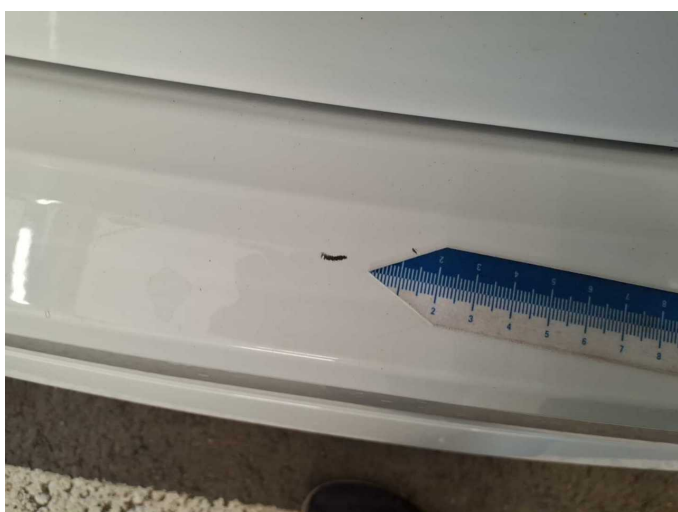
Damage 1: Rear bumper: Rear bumper - Scratched - Smart repair
