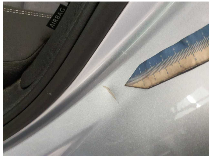
Damage 4: Side panel - rear left side: Sill - Dent / paintcoat damage - Repair and paint
