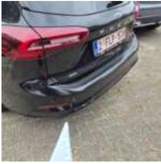
Damage Part Bumper - Rear
