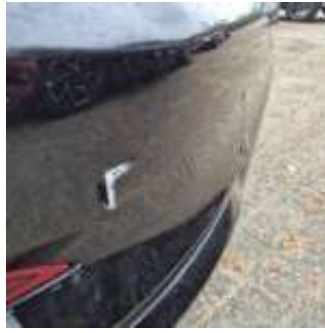
Damage Type small dents / small scratches
