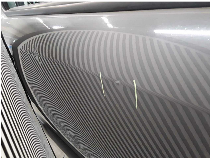
Damage 7: Door - front right side: Door - Dent / paintcoat damage - Repair and paint
