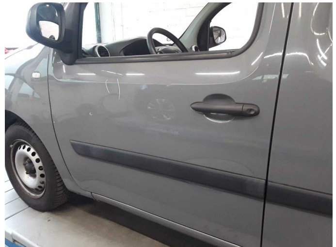
Damage 8: Door - front left side: Door - Dent / paintcoat damage - Repair and paint
