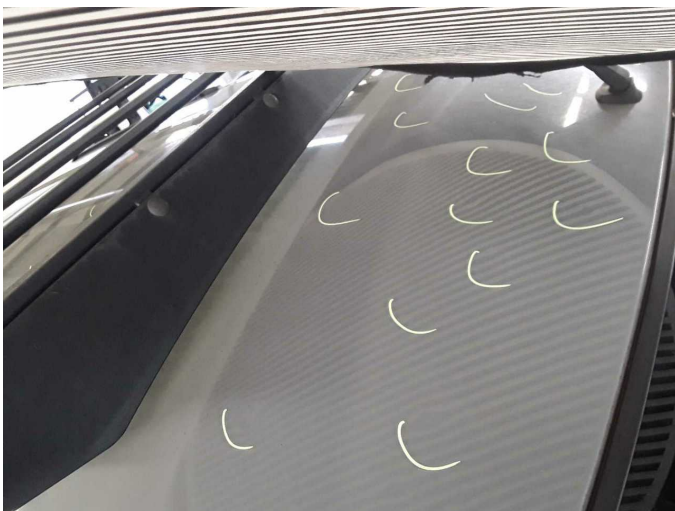
Damage 9: Body: Body - Damage by hail - repair according to calculation
