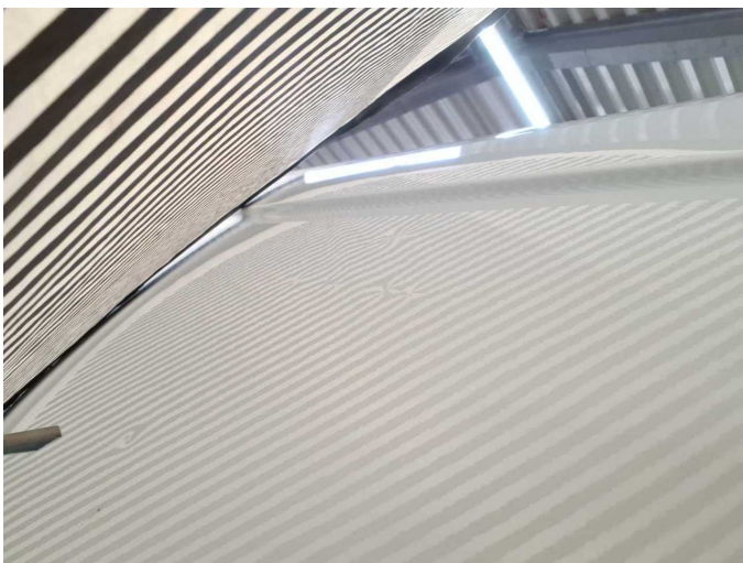
Damage 10: Side panel - rear right side: Side panel - Deformed - Repair and paint
