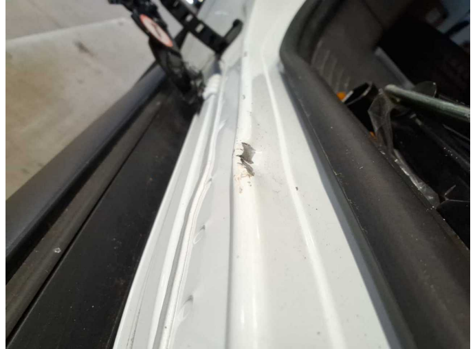
Damage 9: Sill - right side: Sill - Deformed - Repair and paint
