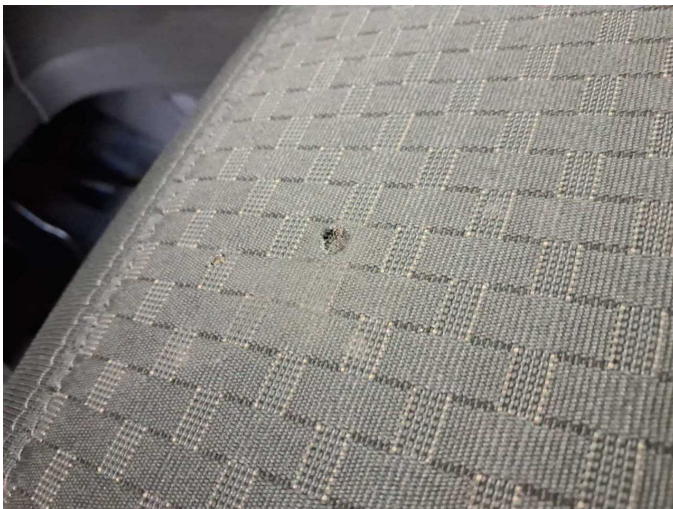
Damage 5: Seat - front: Seat cover - left side - Burn hole (cigarettes) - Smart repair
