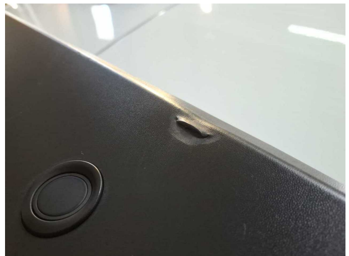
Damage 8: Rear bumper: Rear bumper (unpainted) - Broken / torn - Replace
