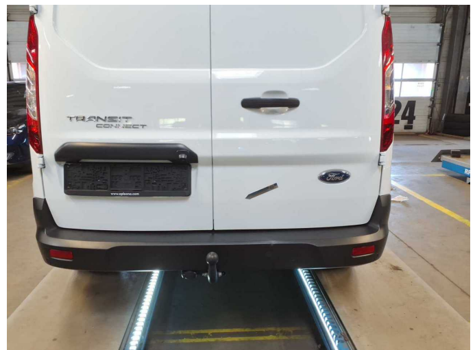
Damage 4: Boot lid / rear door: Rear door - right side - Paint defect - Smart repair
