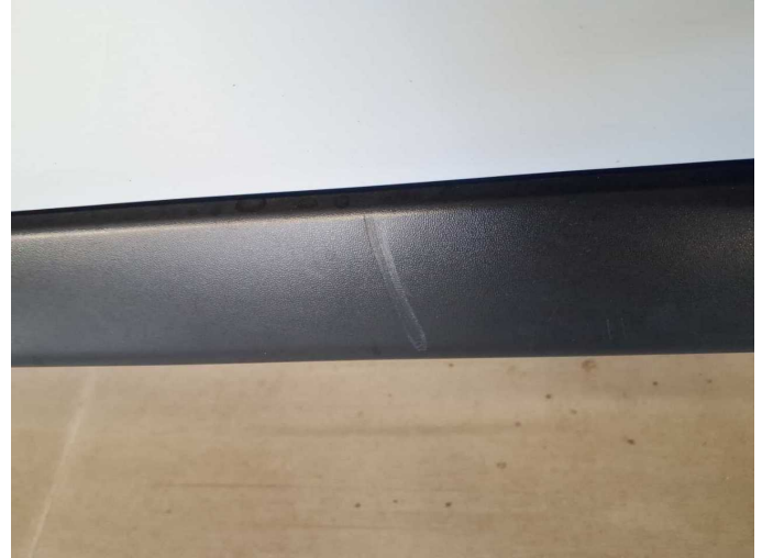
Damage 7: Sill - right side: Trim (Materialabtrag) - Scratched - Replace
