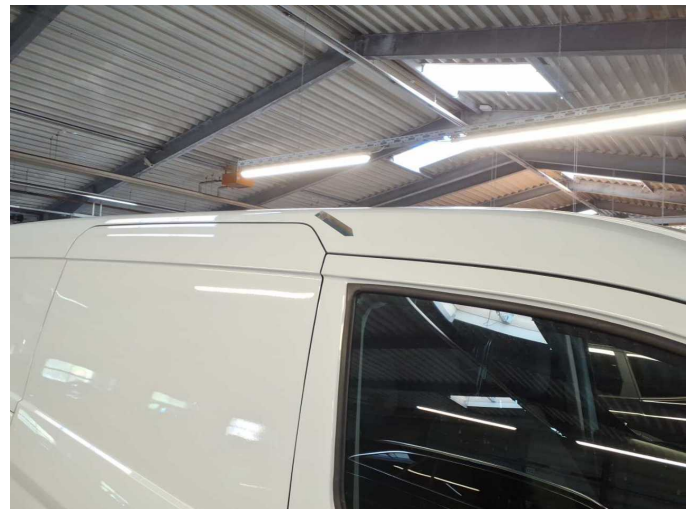
Damage 6: Roof: Roof rail - right side - Dent / paintcoat damage - Smart repair
