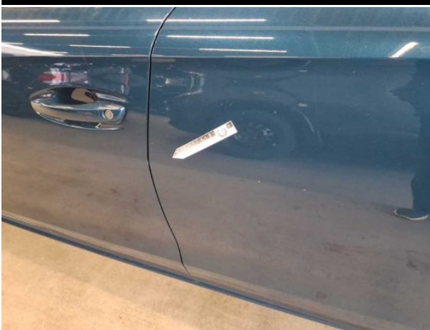
Damage #4: Door - rear left side: Door - Dent / paintcoat damage - Repair and paint
