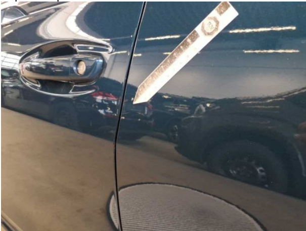
Damage #4: Door - rear left side: Door - Dent / paintcoat damage - Repair and paint
