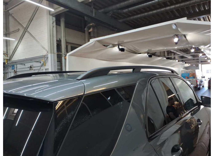
Damage 3: Roof: Roof rail - right side (3x) - dent(s) - Smooth repair work
