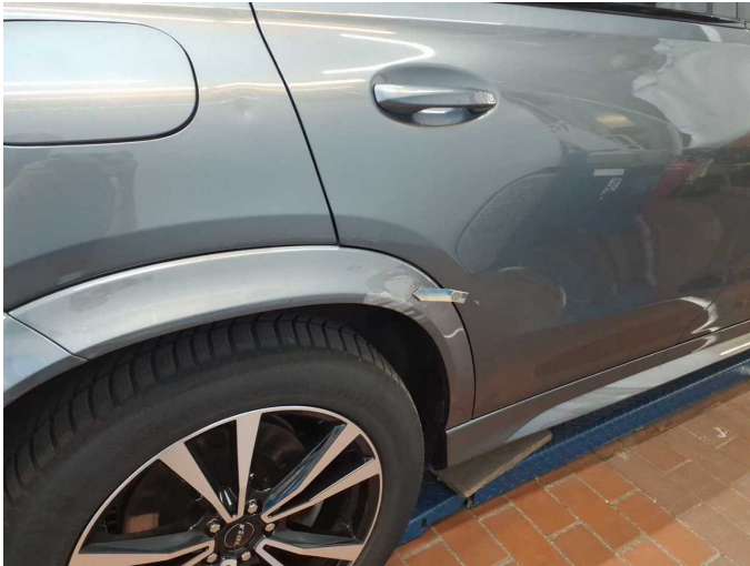
Damage 8: Side panel - rear right side: Wheel well extension - Scratched - Replace
