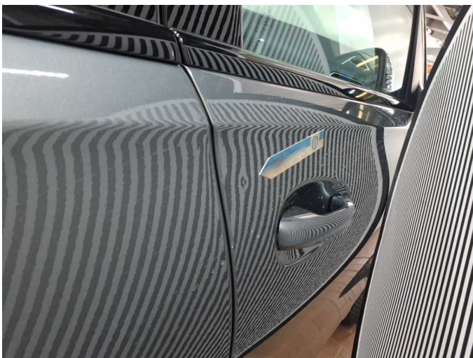
Damage 1: Door - front right side: Door - dent(s) - Smart repair
