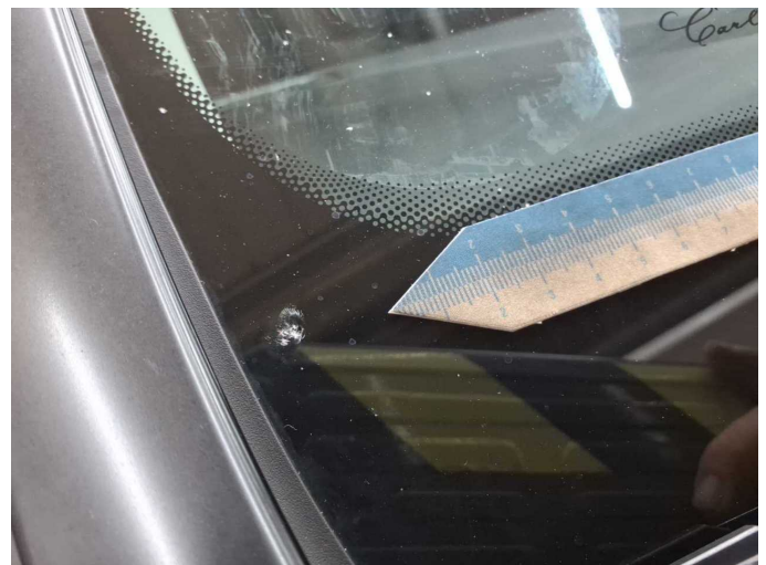
Damage 9: Vehicle glazing: Windscreen (kein Staubschutz) - Stone chips - repair according to calculation
