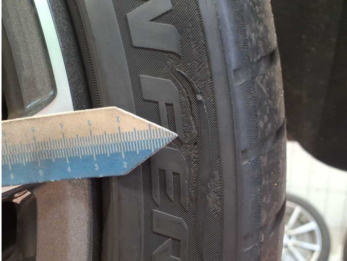
Damage 4: Wheel / tyres: Tyre - rear left side (nicht fahrbereit) - Broken / torn - Replace
