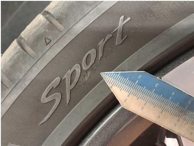
Damage 5: Wheel / tyres: Tyre - front right side (nicht fahrbereit) - Broken / torn - Replace
