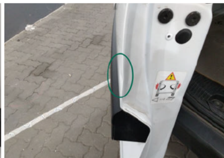
Heckklappe / Kofferraumtür / Mitte Links / Delle
