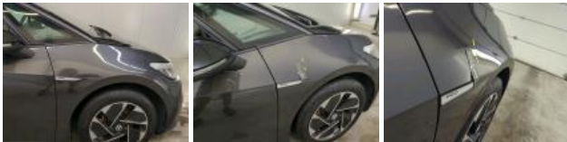
Wing FR, Dent(s), Paintless dent repair
