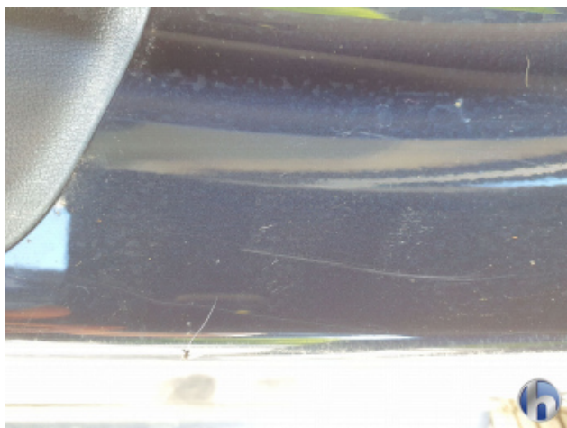
1. Schweller - Links Kratzer - Smart Repair
