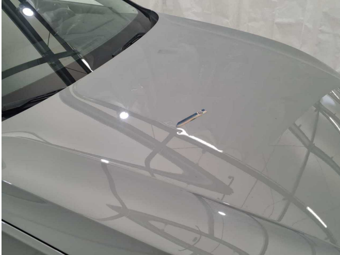
Damage 1: Bonnet: Bonnet - dent(s) - Smooth repair work
