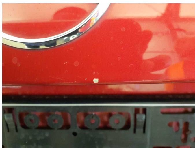
Damage 5: Boot lid / rear door: Boot lid - Scratch(es) - Paint
