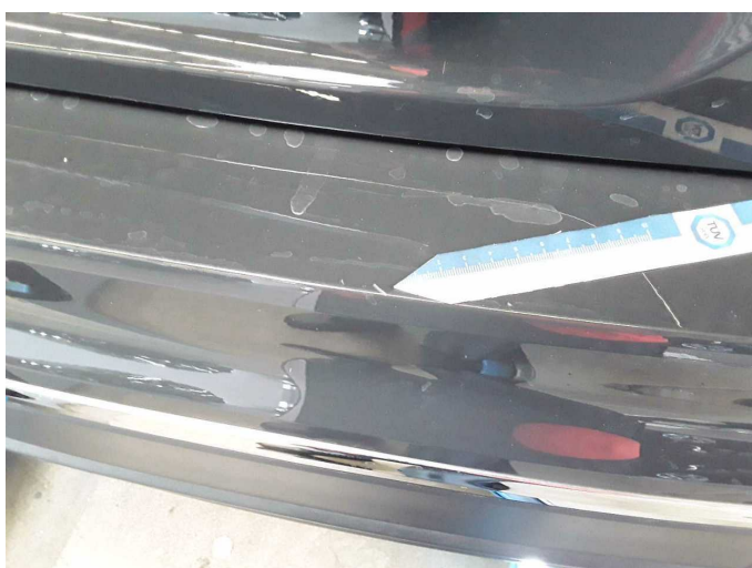
Damage 4: Rear bumper: Rear bumper - Scratch(es) - Paint
