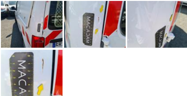
Brand badge F, Missing, Replace
