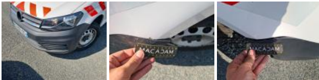
Bumper moulding FL, Unclasp(ed), Dismount/Mount
