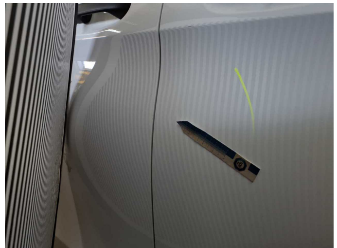
Wear and tear 5: Door - front right side: Door - dent(s) - No deduction
