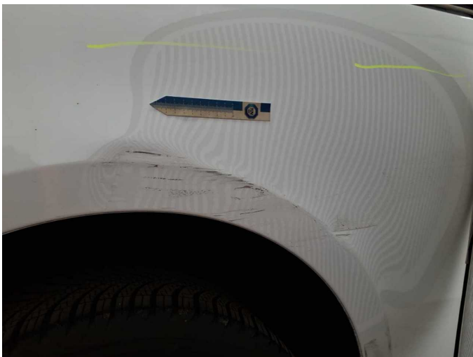
Damage 1: Side panel - rear right side: Side panel (Unterhalb) - Dent / paintcoat damage - Repair and paint
