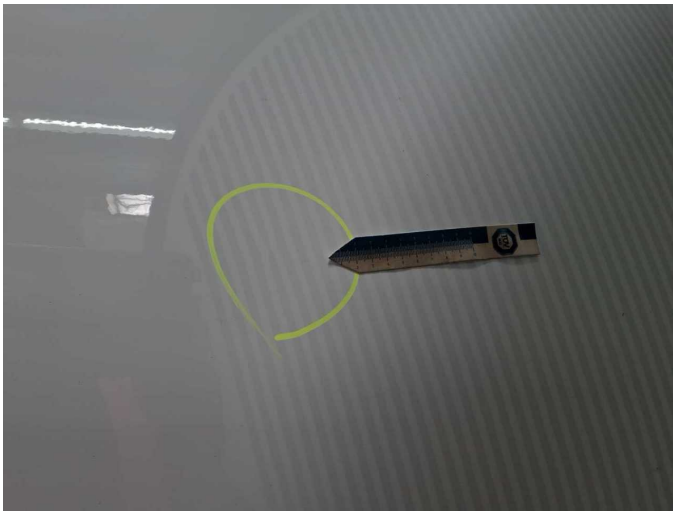
Wear and tear 4: Boot lid / rear door: Rear door - right side - dent(s) - No deduction
