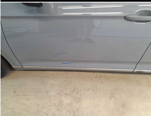
Damage #9: Door - front left side: Door - Scratched - Repair and paint
