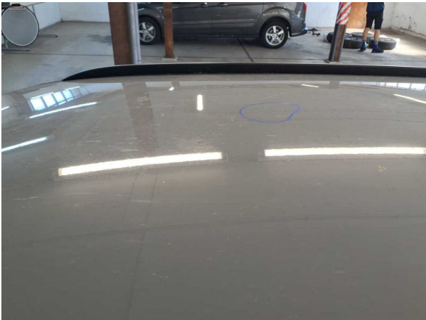
Damage #3: Roof: Roof - dent(s) - Smooth repair work
