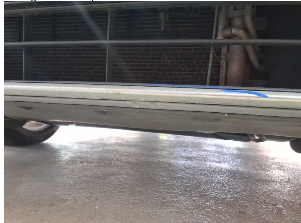
Damage #6: Front bumper: Spoiler - Scratched - Loss in value
