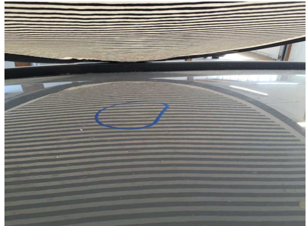
Damage #3: Roof: Roof - dent(s) - Smooth repair work
