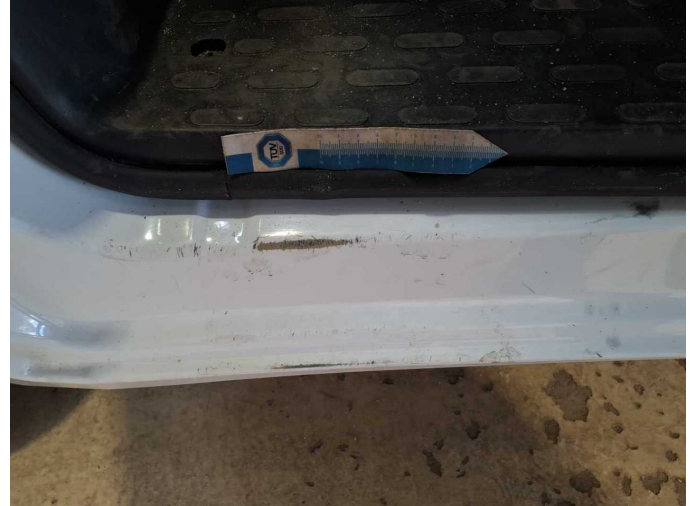
Damage 2: Sill - left side: Sill - Scratch(es) - Smart repair
