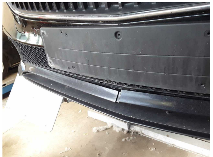
Damage 1: Front bumper: Spoiler - Loose - Un- / install
