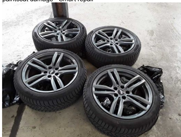
Damage #16: 2nd wheel set: 3 alloy rims - Scratched - Loss in value
