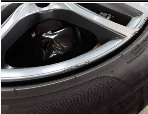
Damage #16: 2nd wheel set: 3 alloy rims - Scratched - Loss in value
