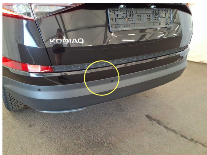
Damage 2: Rear bumper: Rear bumper - Scratch(es) - Paint
