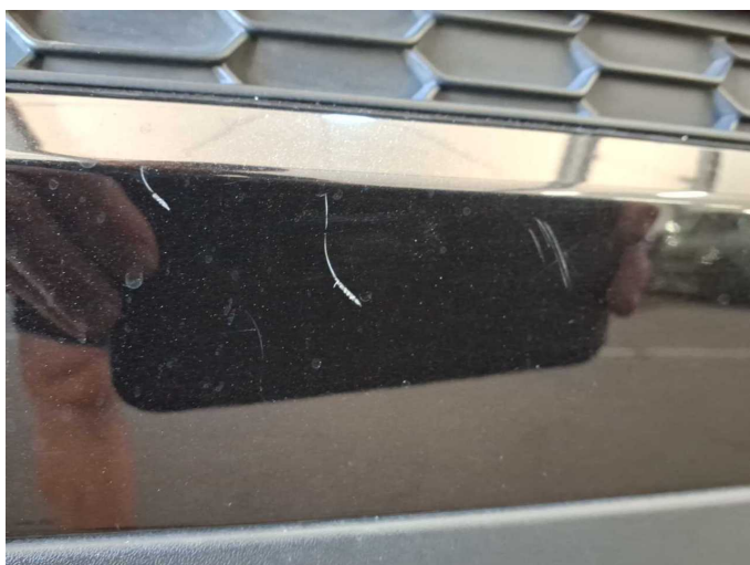
Damage 2: Rear bumper: Rear bumper - Scratch(es) - Paint
