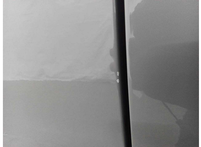
Damage 1: Sliding door, right: Sliding door - Scratch(es) - Smart repair
