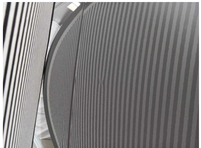
Damage 2: Boot lid / rear door: Rear door - right side (2) - dent(s) - Smooth repair work
