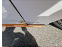
Wing FR, Dent(s) and scratch(es), Repair and paint (complete)
