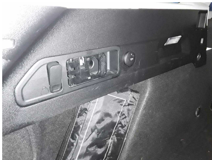
Damage 1: Seat - front: Lever seat adjustment (Hinten) - Damaged - Replace
