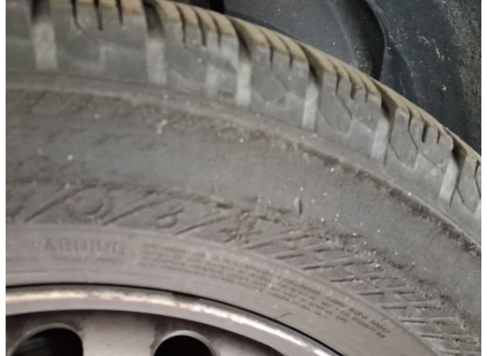
Damage 5: Wheel / tyres: Tyre - front right side (225,65,16,g) - Broken / torn - Replace
