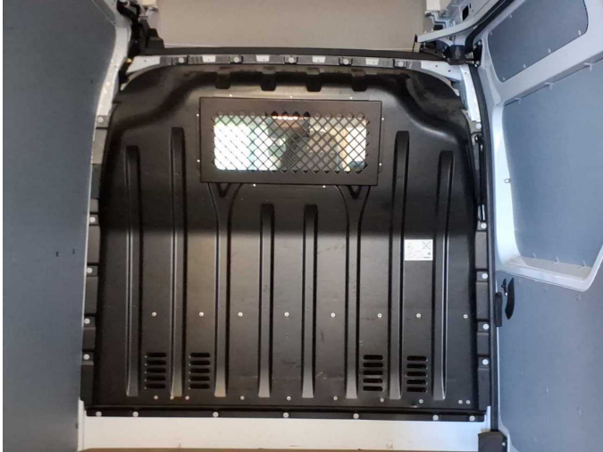
Wear and tear 1: Body: Partition wall - Dent / paintcoat damage - No deduction
