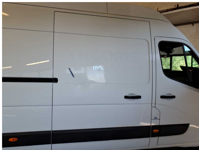
Damage 12: Sliding door, right: Sliding door - Dent / paintcoat damage - Repair and paint
