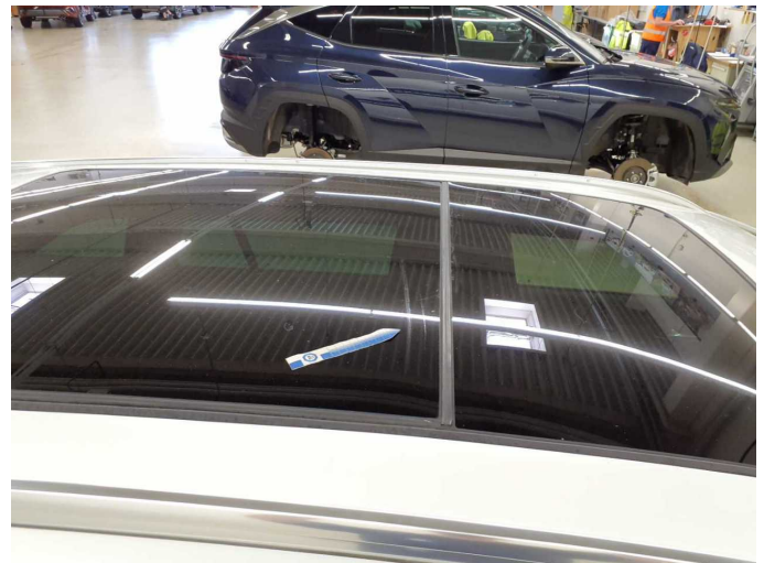
Damage 7: Roof: Sun roof / glass - Scratched - Replace
