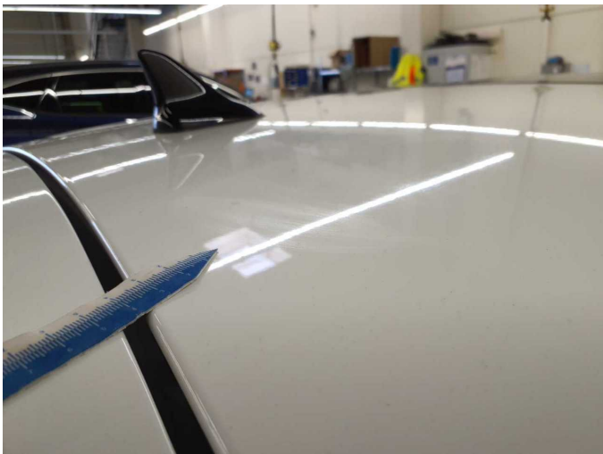
Damage 3: Body: Body - Scratched - Conditioning
