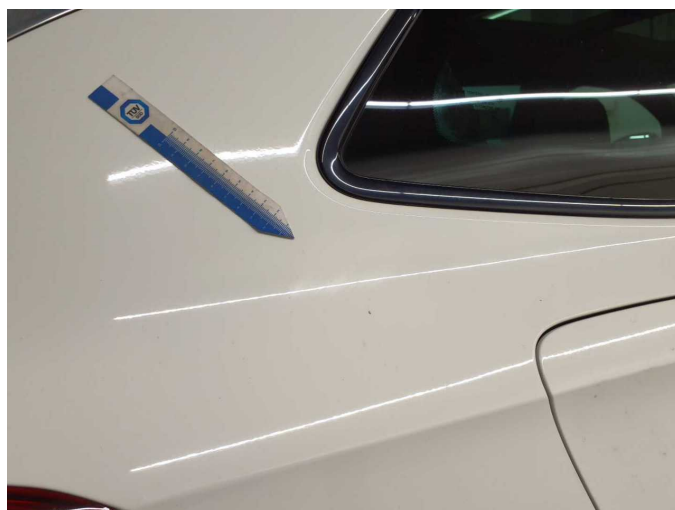
Damage 3: Body: Body - Scratched - Conditioning
