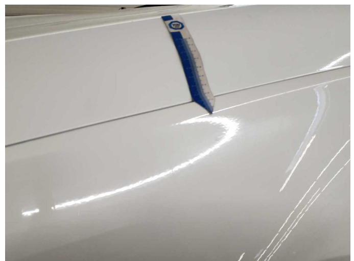
Damage 3: Body: Body - Scratched - Conditioning
