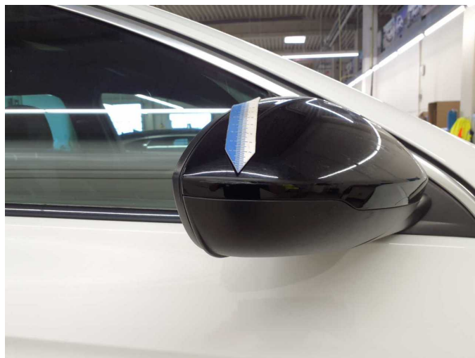
Wear and tear 1: Wing mirror - right side: Cap - Scratched - No deduction
