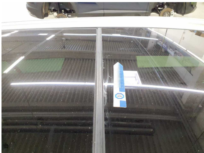
Damage 7: Roof: Sun roof / glass - Scratched - Replace
