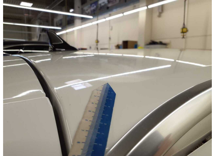
Damage 3: Body: Body - Scratched - Conditioning
