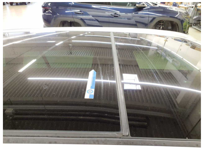
Damage 7: Roof: Sun roof / glass - Scratched - Replace
