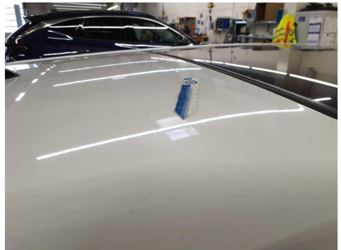
Damage 3: Body: Body - Scratched - Conditioning
