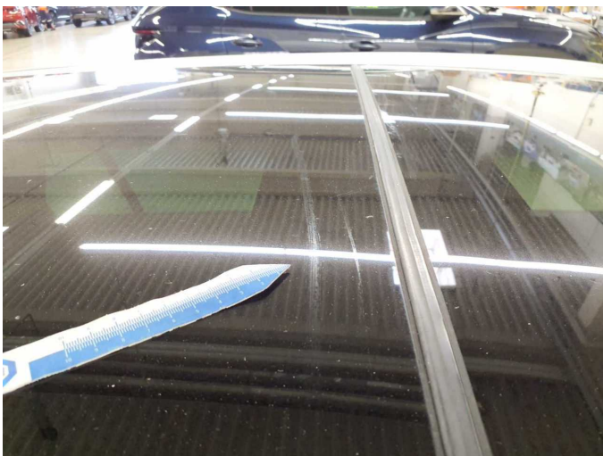
Damage 7: Roof: Sun roof / glass - Scratched - Replace
