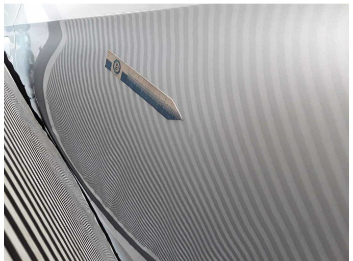
Damage 2: Door - rear left side: Door - Dent / paintcoat damage - Smart repair
