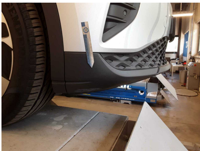
Damage 4: Front bumper: Spoiler - Scratched - Replace
