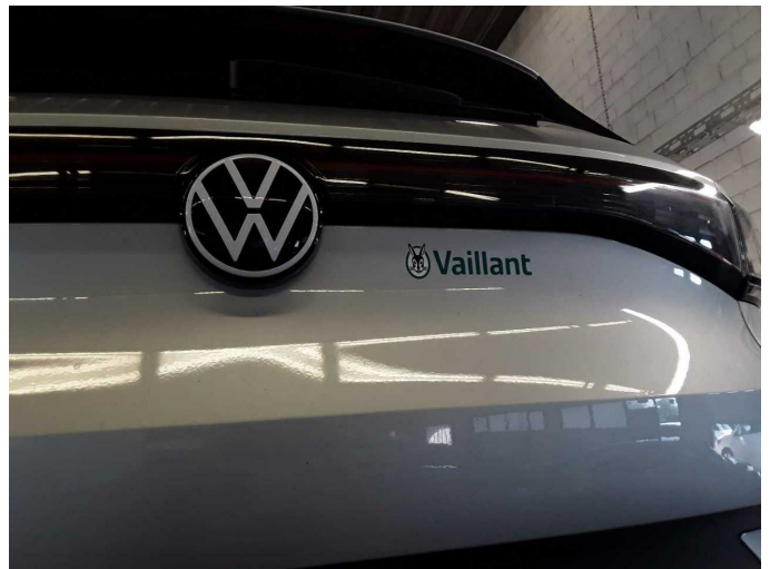
Damage 1: Body: Body - Glued / labelled - De-glue / neutralise
