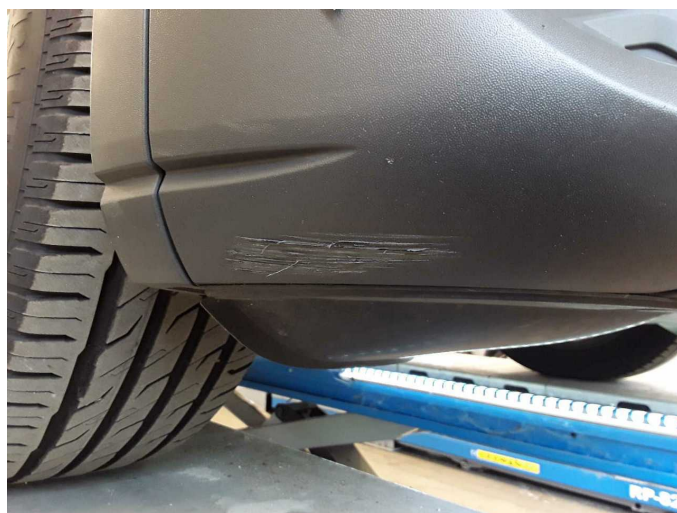
Damage 4: Front bumper: Spoiler - Scratched - Replace
