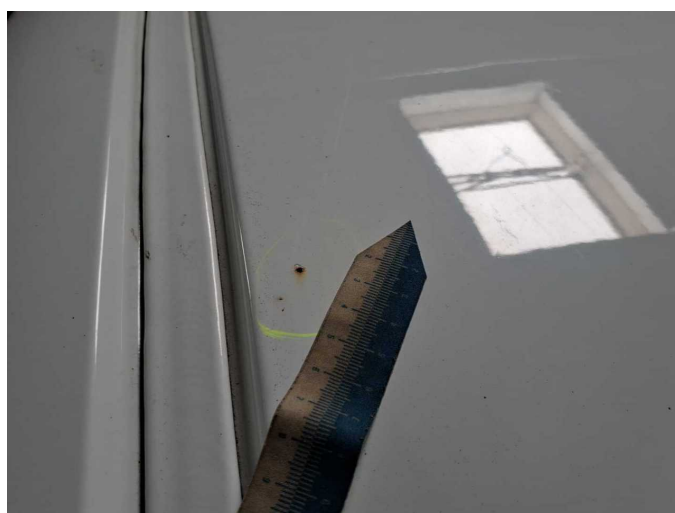
Damage 6: Roof: Roof - Dent / paintcoat damage - Repair and paint
