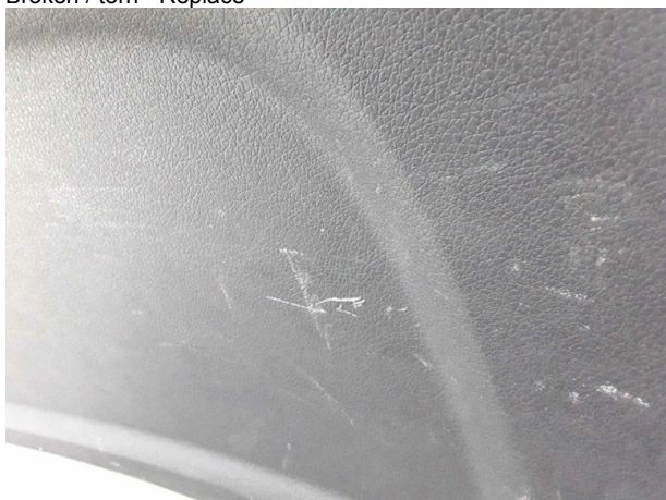
Damage #11: Trim / covers: Boot lid - interior trim - Scratched - Replace
