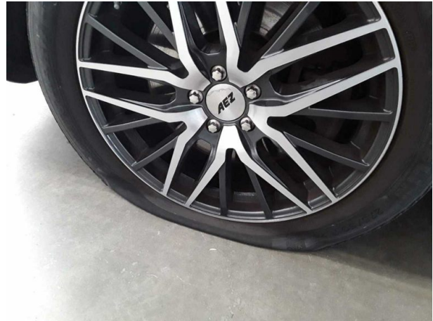
Damage #2: Wheel / tyres: Alloy rim - front left side (Reifen platt; Felge prüfen) - Specify findings - No deduction
