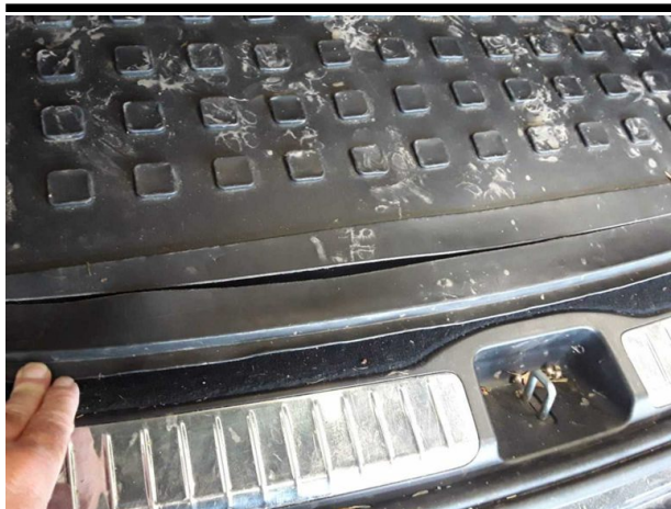
Damage #9: Trim / covers: Boot lining (Ladeboden Formmatte) - Broken / torn - Replace
