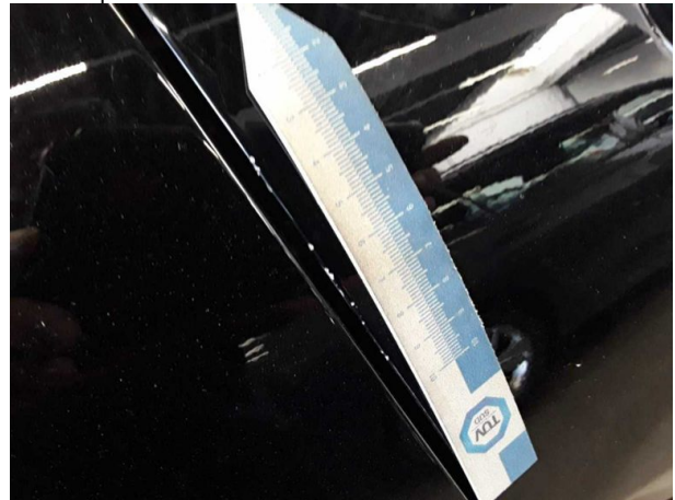
Damage #7: Door - rear right side: Door edge - Scratched - Smart repair
