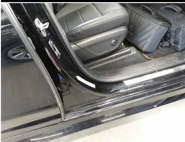
Damage #6: Sill - right side: Sill - Dent / paintcoat damage - Smart repair
