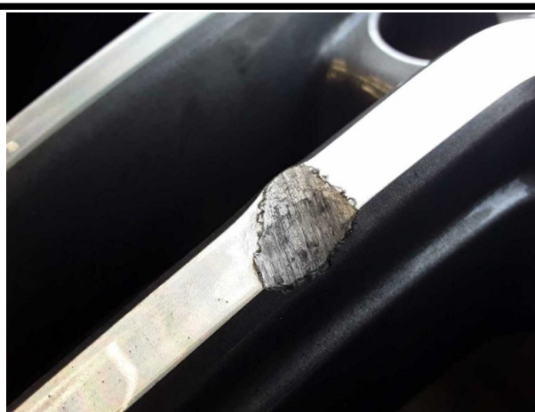
Damage #10: 2nd wheel set: 1 alloy rim - Deformed - Loss in value
