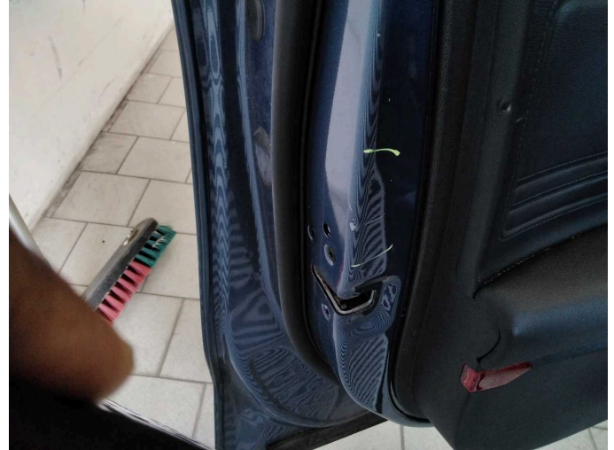
Damage 7: Door - front left side: Door (Innen) - Dent / paintcoat damage - Smart repair
