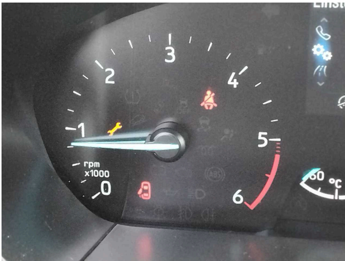
Damage 8: Instrument panel: Indicator light - on - Perform diagnosis
