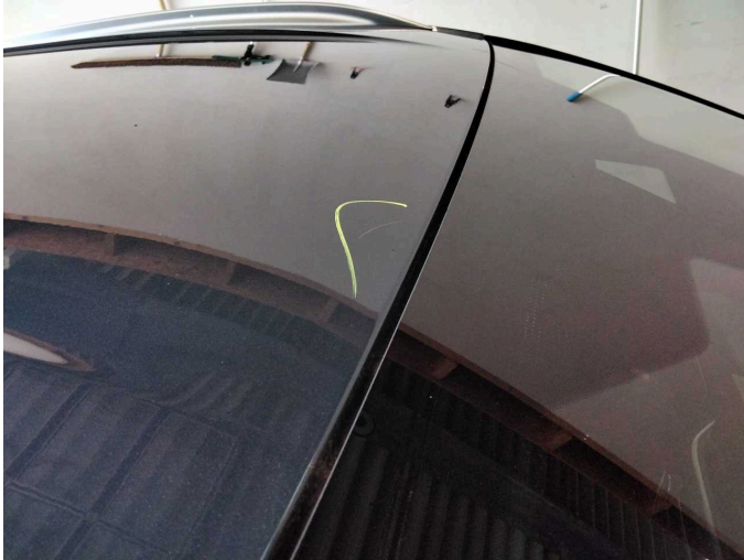
Damage 2: Roof: Roof - Scratch(es) - Smart repair
