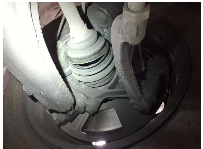
Damage 2: Drive train: Sleeve prop shaft - front right side - Broken / torn - Replace
