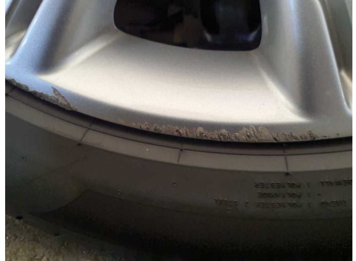
Damage 7: Wheel / tyres: Alloy rim - rear right side (- Materialabtrag) - Scratched - Replace
