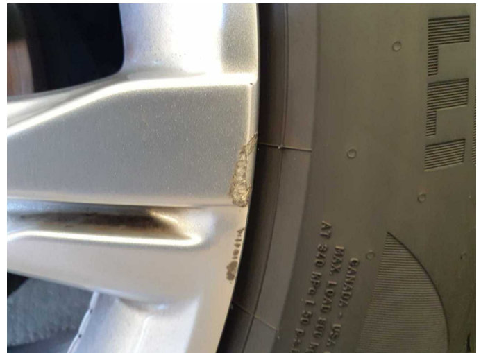
Damage 6: Wheel / tyres: Alloy rim - rear left side (- Materialabtrag) - Scratched - Replace
