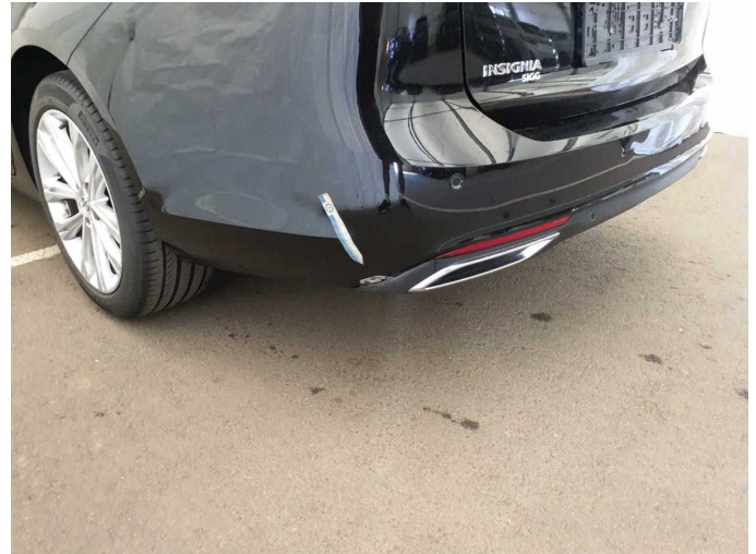
Damage 9: Rear bumper: Rear bumper - Broken / torn - Replace
