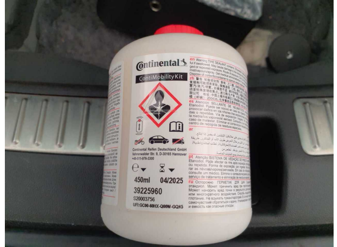
Damage 1: Equipment: Tirefit filler - Expired - Replace
