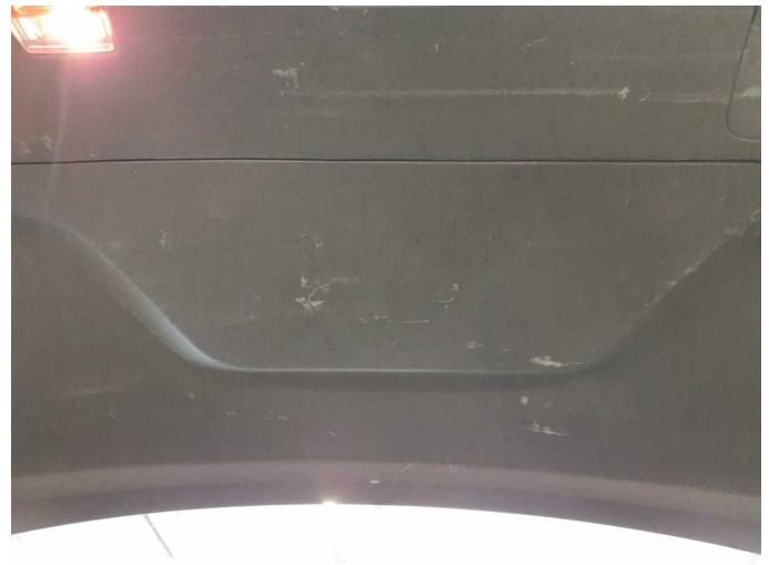
Damage 1: Trim / covers: Boot lid - interior trim - Scratch(es) - Loss in value
