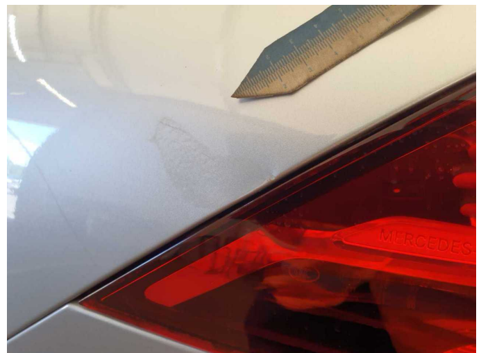
Damage 9: Side panel - rear left side: Side panel - Dent / paintcoat damage - Repair and paint
