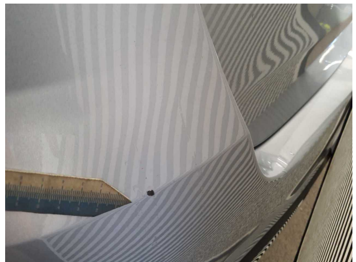
Damage 7: Rear bumper: Rear bumper - Scratch(es) - Paint
