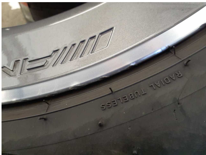
Damage 10: 2nd wheel set: 2 alloy rims (Materialabtrag) - Scratched - repair according to calculation
