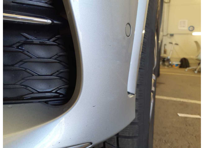
Damage 8: Front bumper: Front bumper - Scratch(es) - Paint
