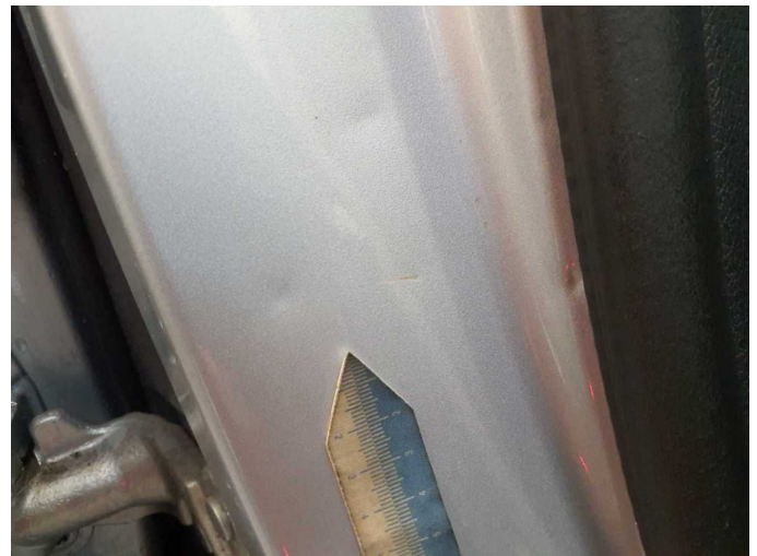
Damage 3: Sill - right side: Sill - Dent / paintcoat damage - Smart repair
