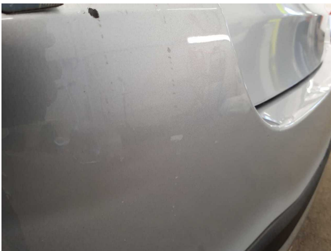
Damage 7: Rear bumper: Rear bumper - Scratch(es) - Paint
