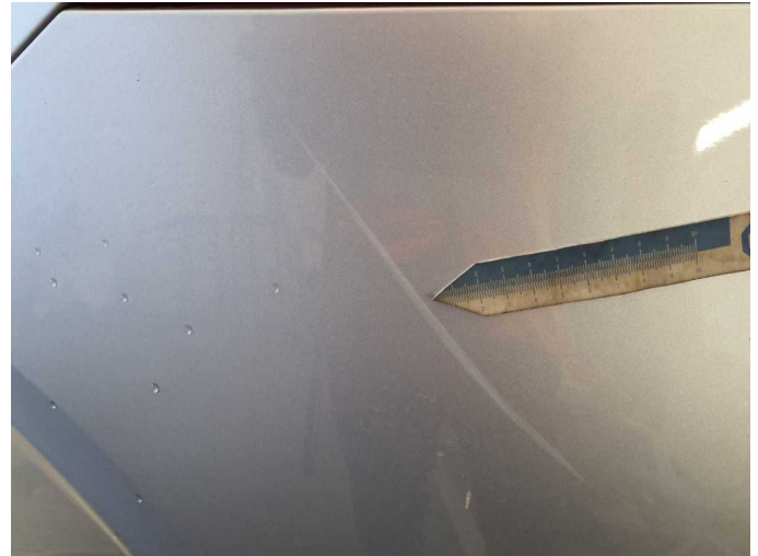
Damage 7: Rear bumper: Rear bumper - Scratch(es) - Paint
