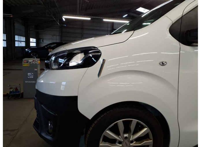
Damage 8: Mudguard - left side: Mudguard - left side - Deformed - Repair and paint
