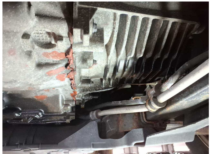
Damage 3: Engine: Engine (+ Getriebe) - Leaking - Perform diagnosis
