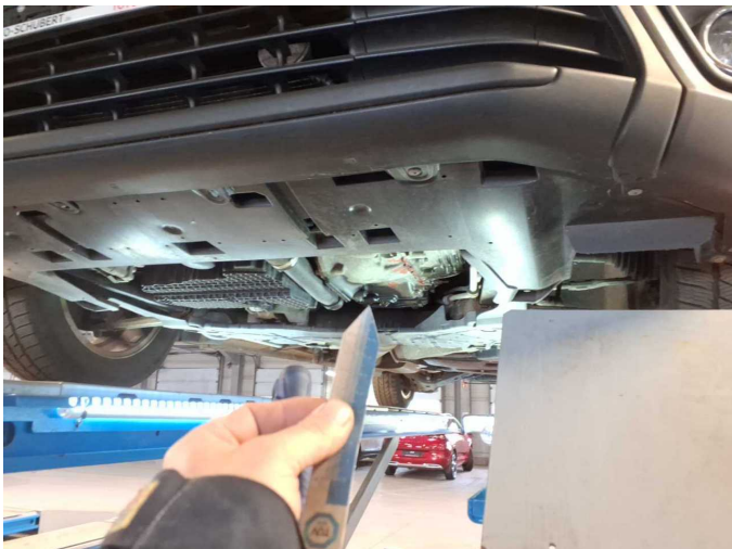
Damage 3: Engine: Engine (+ Getriebe) - Leaking - Perform diagnosis
