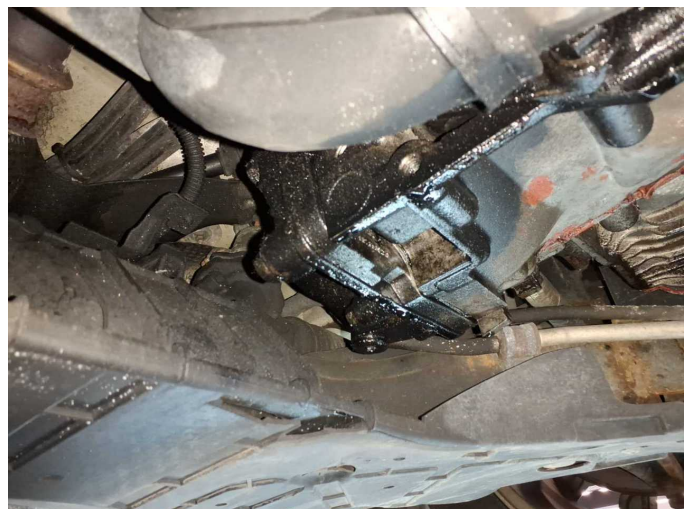
Damage 3: Engine: Engine (+ Getriebe) - Leaking - Perform diagnosis
