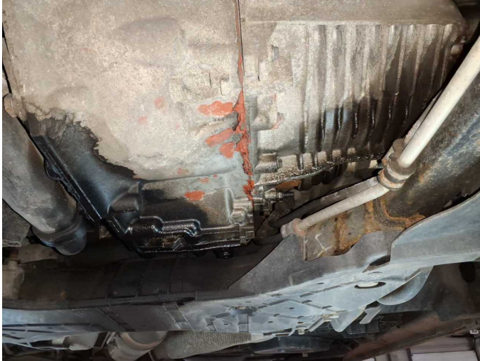
Damage 3: Engine: Engine (+ Getriebe) - Leaking - Perform diagnosis
