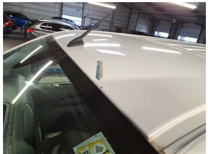
Damage 10: Roof: Roof (Korrosion) - Stone chips - Paint
