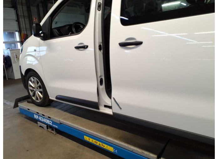
Damage 11: Sliding door - left side: Sliding door (Korrosion) - Scratched - Repair and paint
