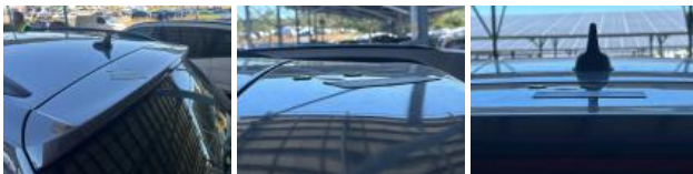
Roof, Hail damage, Repair and paint (complete)
