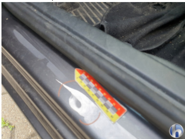
2. Türeinstieg Vorne - Links 1 Delle - Smart Repair
