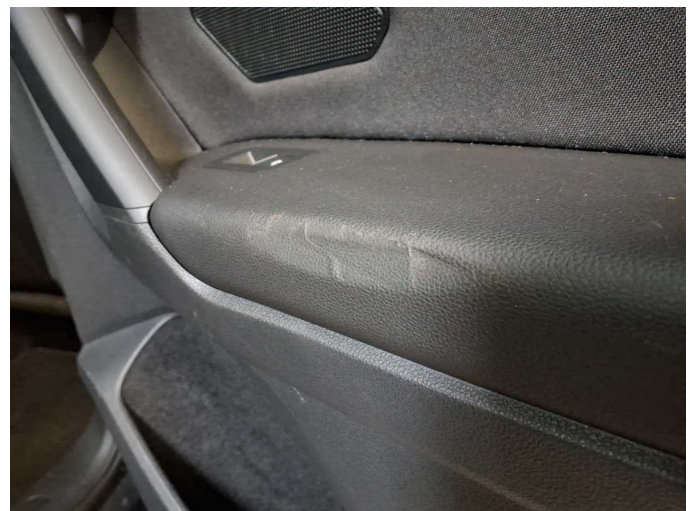
Damage 2: Door - rear right side: Door handle - inside - Deformed - Replace
