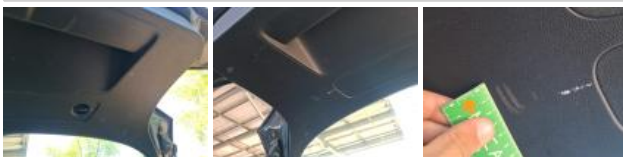
Boot lid covering R, Scratch(es), Replace
