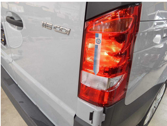
Damage 5: Tail light: Tail lamp - right side - Scratch(es) - Replace
