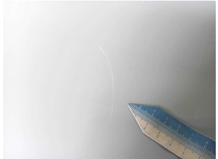
Damage 6: Bonnet: Bonnet - Scratch(es) - Paint
