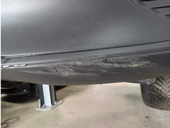
Damage 8: Front bumper: Front bumper - Scratch(es) - Replace
