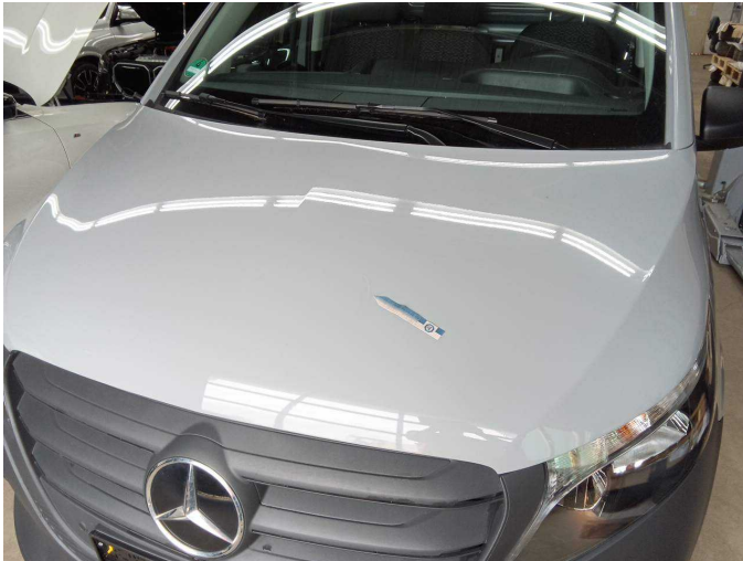
Damage 6: Bonnet: Bonnet - Scratch(es) - Paint
