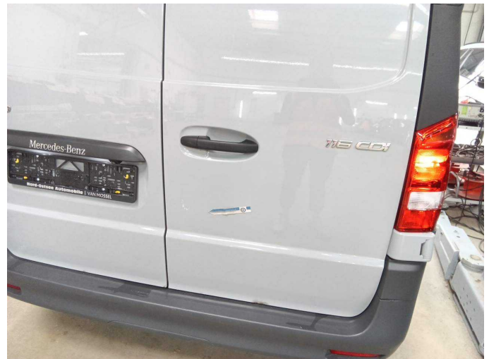
Damage 7: Boot lid / rear door: Rear door - right side - Scratch(es) - Paint
