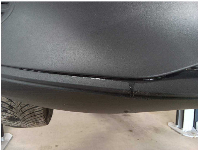
Damage 8: Front bumper: Front bumper - Scratch(es) - Replace
