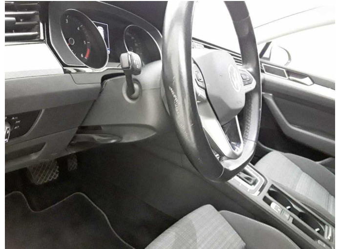
Damage 5: Steering system: Steering wheel sheath - Scratched - Smart repair
