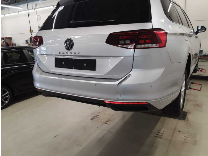
Damage 9: Rear bumper: Rear bumper - Scratched - Paint
