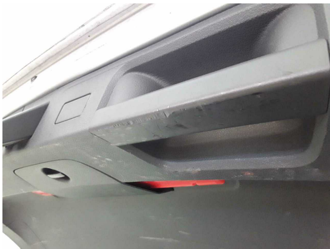
Damage 7: Boot lid / rear door: Trim - standard - lower - Scratched - Replace
