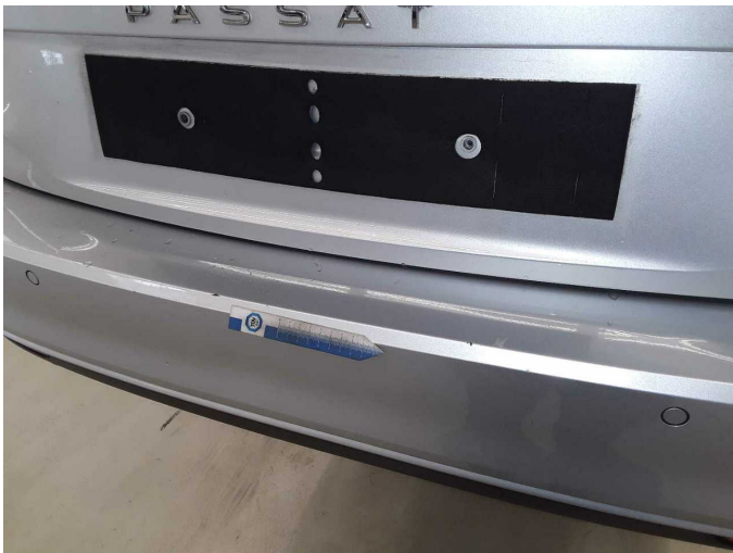
Damage 9: Rear bumper: Rear bumper - Scratched - Paint
