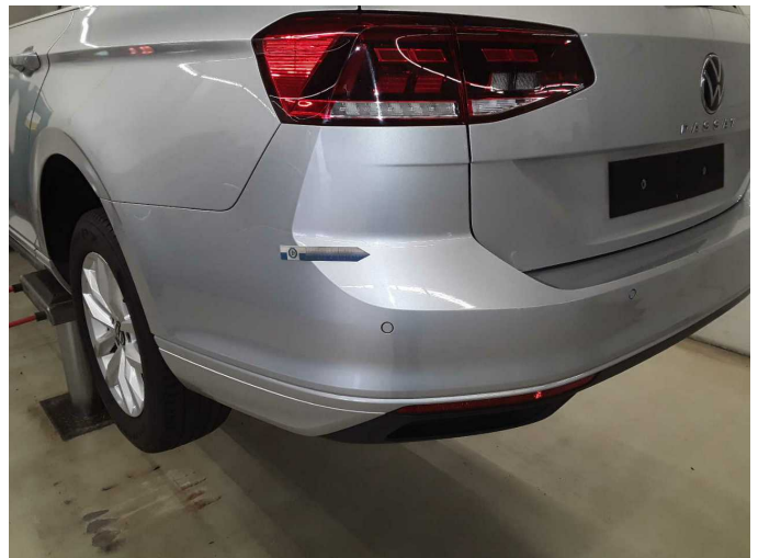
Damage 9: Rear bumper: Rear bumper - Scratched - Paint
