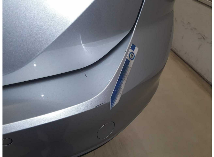
Damage 9: Rear bumper: Rear bumper - Scratched - Paint
