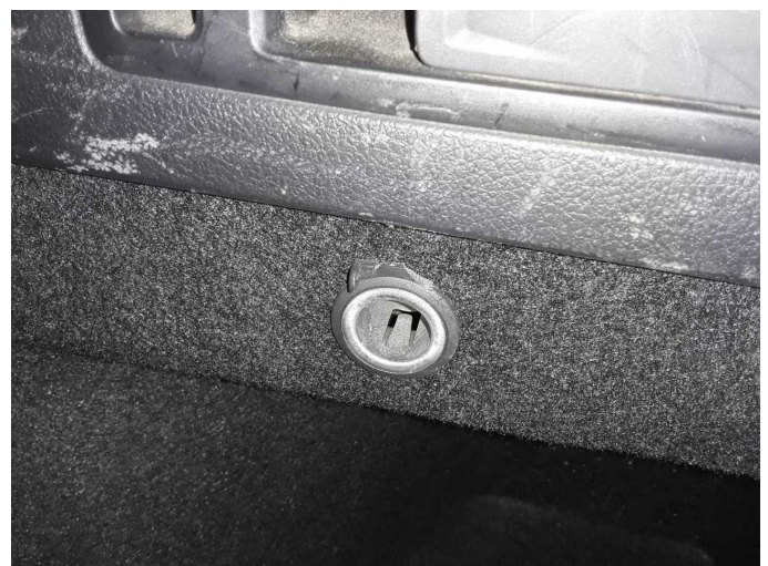
Damage 8: Trim / covers: Cargo area - lining - right side (Steckdosendeckel) - Broken / torn - Replace
