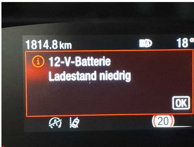
Damage 1: Electrical system: Battery - Empty - Perform
