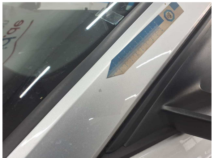
Damage 2: Body: A-pillar - left side - Stone chips - Smart repair
