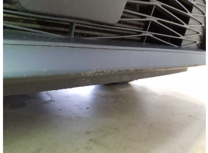
Damage 13: Front bumper: Front bumper (+ Spoiler erneuern) - Dent / paintcoat damage - Paint
