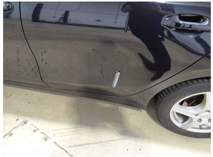
Damage 20: Door - rear left side: Door (Spachtel eingefallen) - Unprofessionally repaired - Repair and paint
