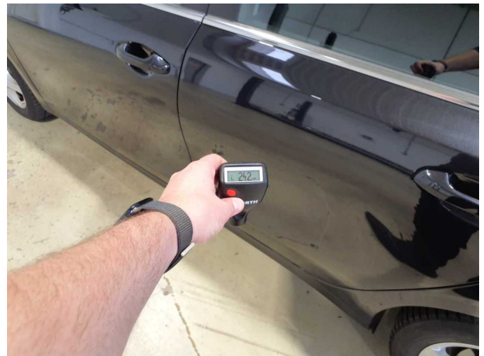
Repainting 1: Door - rear left side
