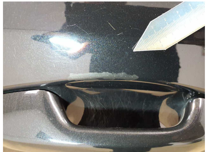
Damage 14: Door - front right side: Door (Lackstift) - Paint defect - Paint
