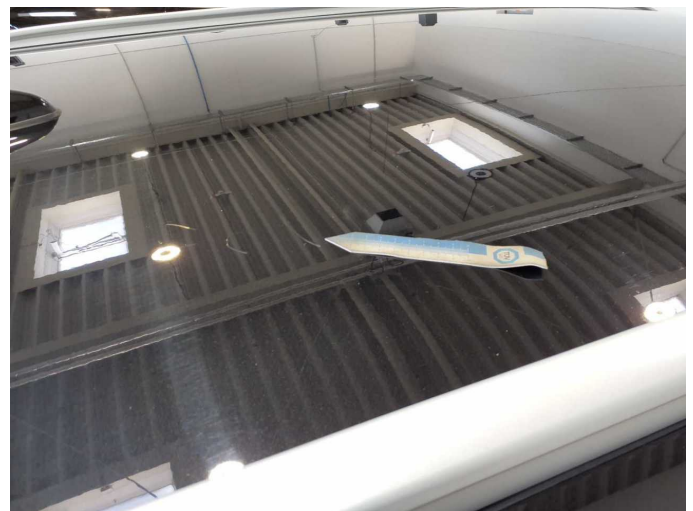
Damage 15: Roof: Roof - Scratch(es) - Paint
