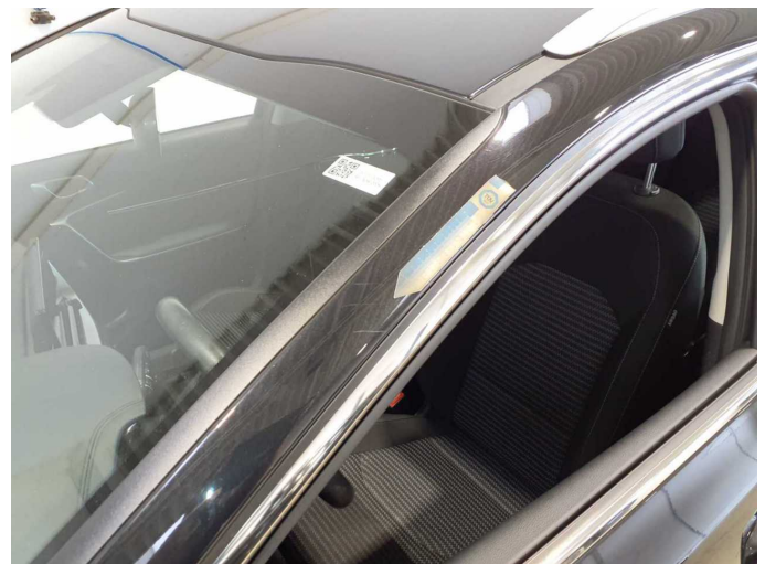
Damage 6: Body: A-pillar - left side - Scratch(es) - Smart repair
