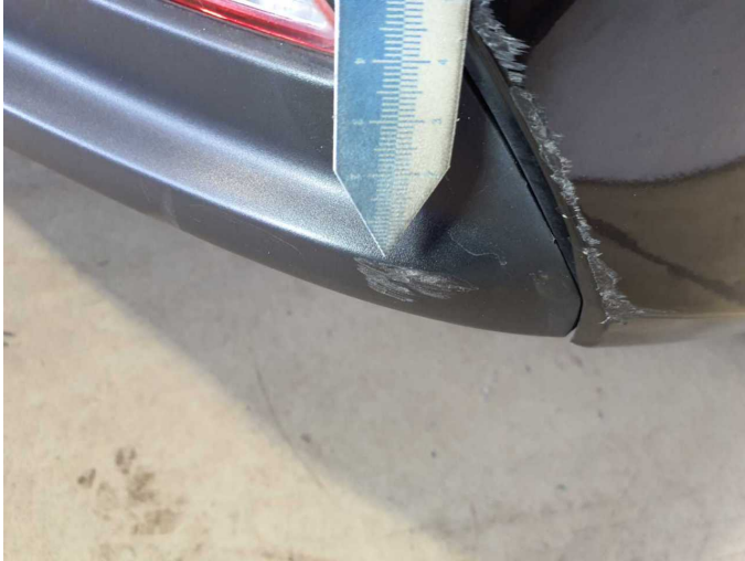
Damage 9: Rear bumper: Spoiler - Scratch(es) - Replace
