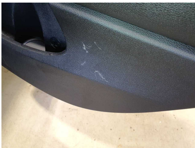
Damage 8: Trim / covers: Door trim - rear right side - Scratch(es) - Loss in value
