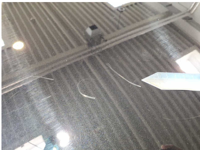
Damage 15: Roof: Roof - Scratch(es) - Paint
