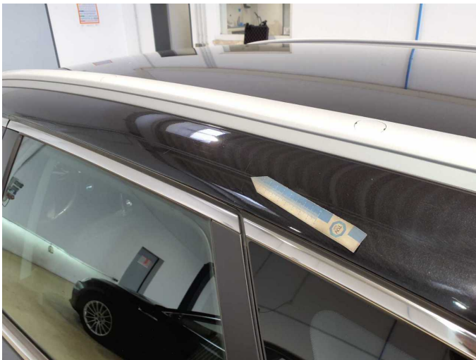
Damage 5: Roof: Roof rail - left side - Scratch(es) - Smart repair
