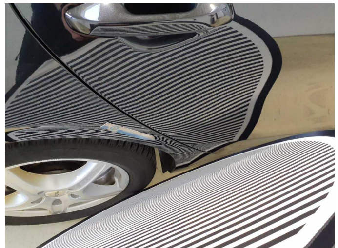
Damage 18: Side panel - rear right side: Side panel (Einschlüsse) - Paint defect - Repair and paint
