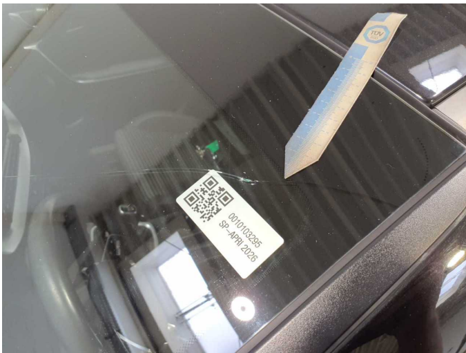
Damage 19: Vehicle glazing: Windscreen - Broken / torn - Replace
