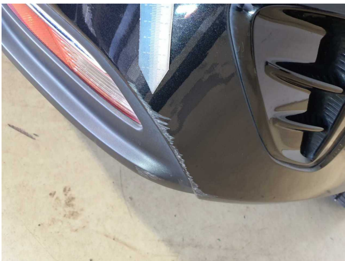
Damage 11: Rear bumper: Rear bumper - Scratch(es) - Paint
