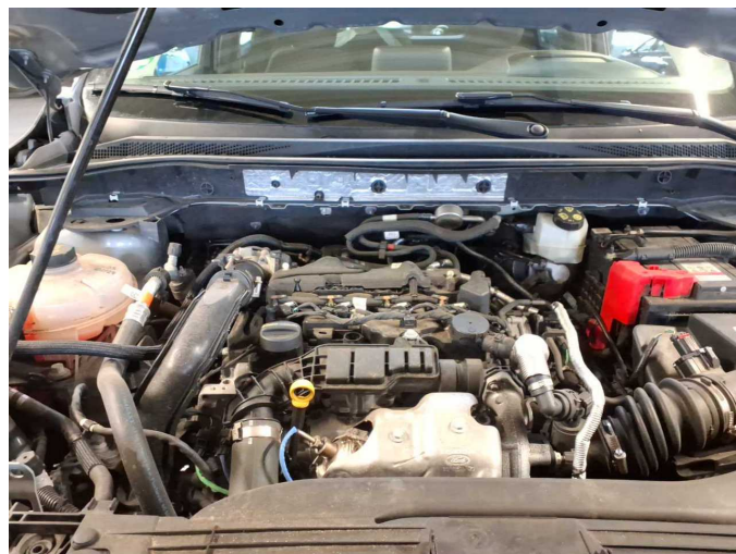
Missing part 1: Engine: Engine cover - Missing - Replace
