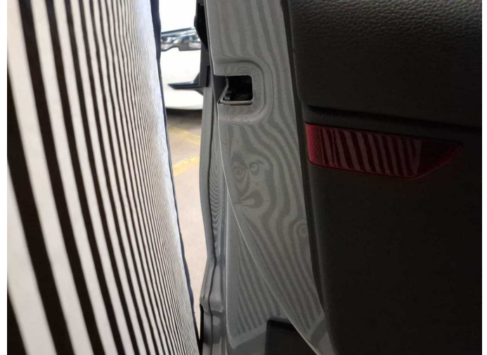
Damage 7: Door - front left side: Door (Innen) - dent(s) - Smooth repair work
