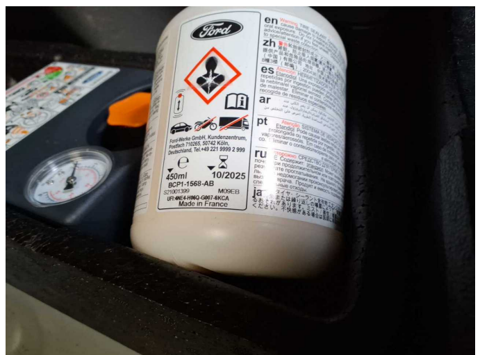
Damage 3: Equipment: Tirefit filler - Expired - Replace
