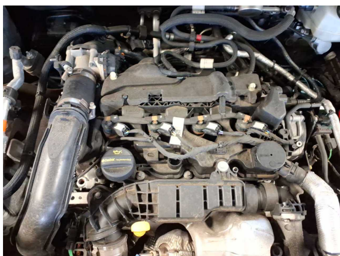
Missing part 1: Engine: Engine cover - Missing - Replace
