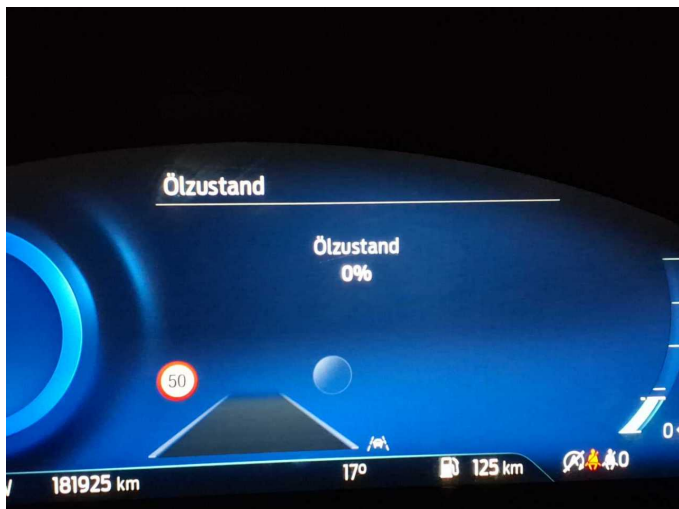
Damage 10: Misc.: Inspection / maintenance - Due - Perform
